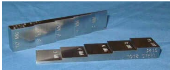
5-step Thickness Reference Block
