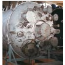
Figure 1: Container made of highly corrosion resistant duplex stainless steel
