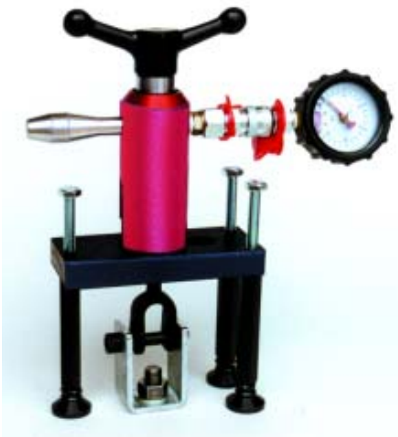
Standard Anchor Test with Bolt Test Adaptor
