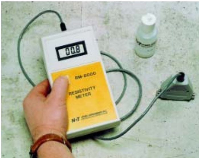
OhmCorr Resistivity Meter
