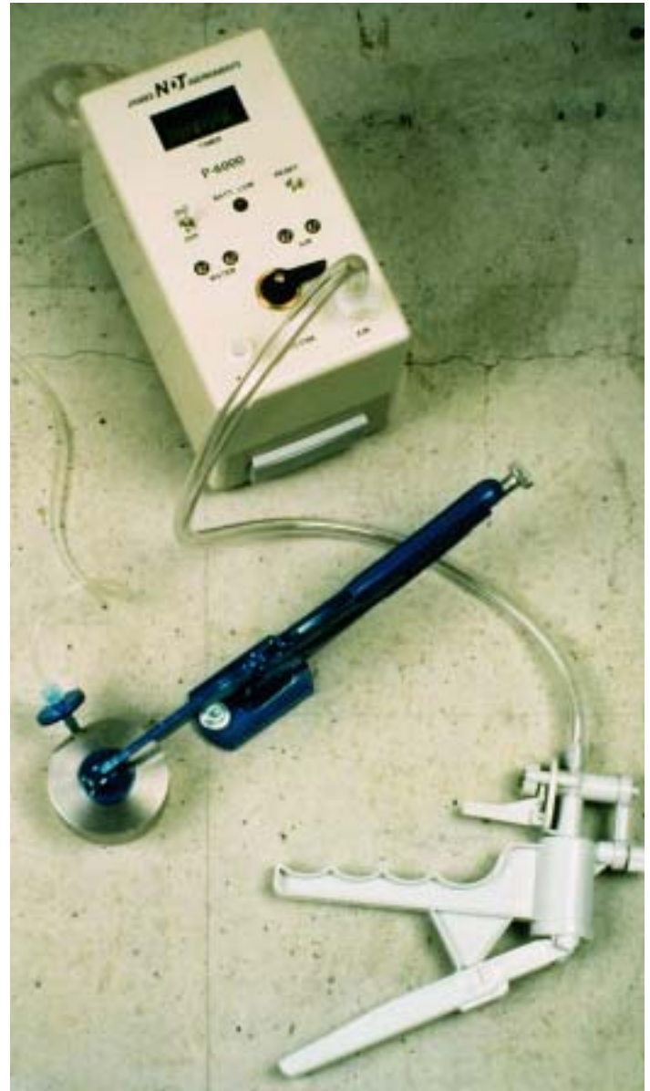
Surface Air Permeability Test
